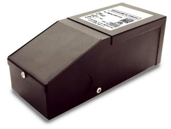
KLUS - MD-60-24 is the most compact LED driver on the market with a magnetic transformer core. It is equipped with two auto-reset breakers, one on the input and one on the output, which protect both the load and driver. The driver is encased in a coated metal box that includes 2 knock-outs, one on each side, to enable easy installation that complies with electrical code requirements.
