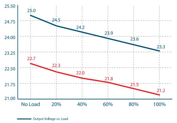
Output Voltage With a Typical Dimmer
